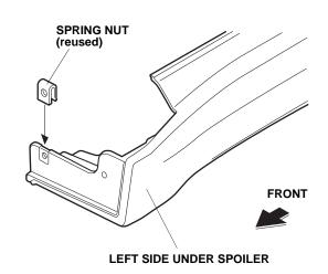
11. Install three spring nuts removed in step 6 on the rear of the left side under spoiler.
