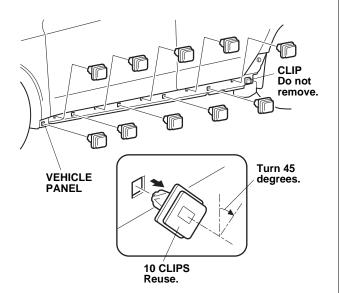
8. Using the clip remover, remove the pin from the grommet.
