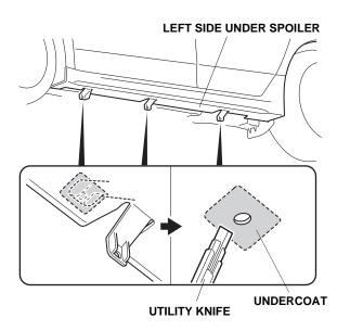
18. Under the vehicle, install the three clips into the left side under spoiler.
