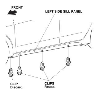
3. Slide the left side sill panel rearward to release the clips, and pull it out to remove the panel.
