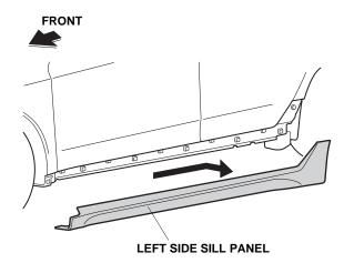
4. Gently lift up the left front inner fender, then slide the left side sill inner trim forward, and pull it toward you to remove it.
