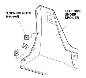
12. Install the ten clips removed in step 7 to the lower clip holders on the left side under spoiler.
