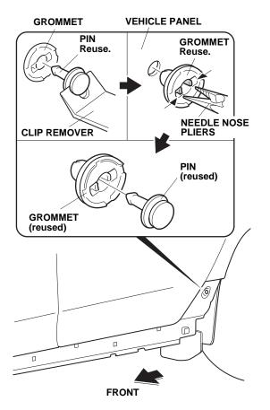
9. Using needle nose pliers, remove the round grommet from the vehicle panel. Reassemble the pin and grommet to be used later.
