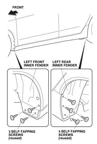
20. Repeat steps 1 thru 19 to install the right under spoiler to the right side of the vehicle.
